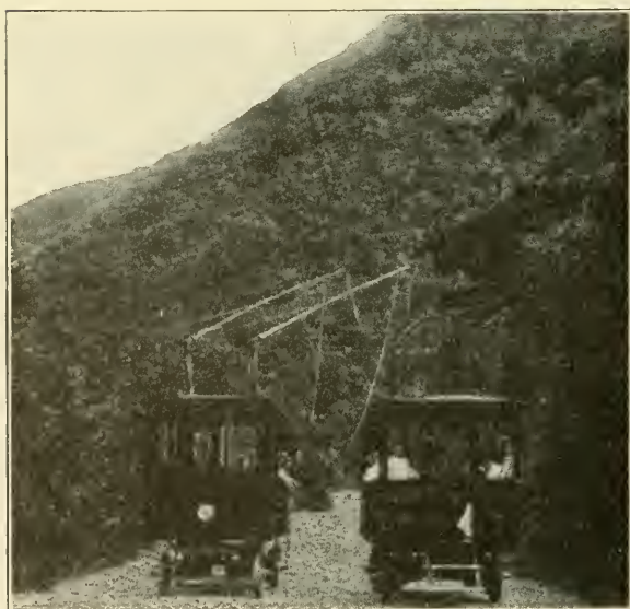
Fig. 23. Cars Passing in Laurel Cañon Drive. Car at Right Is Coasting with Trolleys Down
